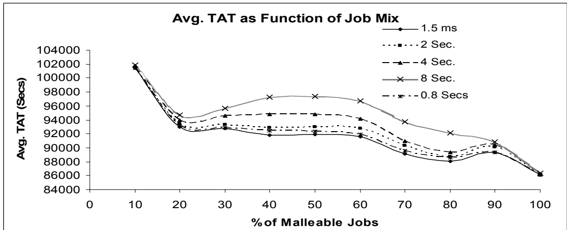
Figure 6.12 Impact of negotiation cost on avg. TAT. Flexibility range: 2- 128, adaptation cost: 2ms
